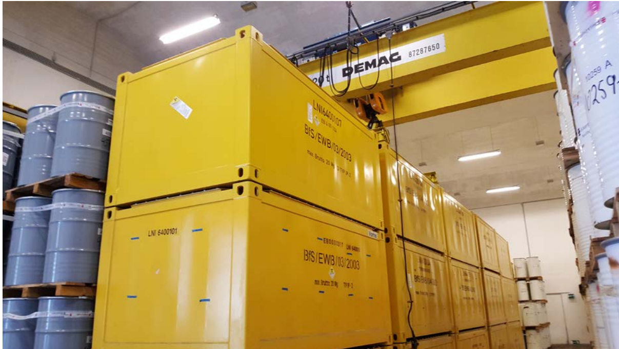
Fig. 5: Konrad Containers Type IV, conditioned for the repository, at Leese (Photo: J. Bluth)
