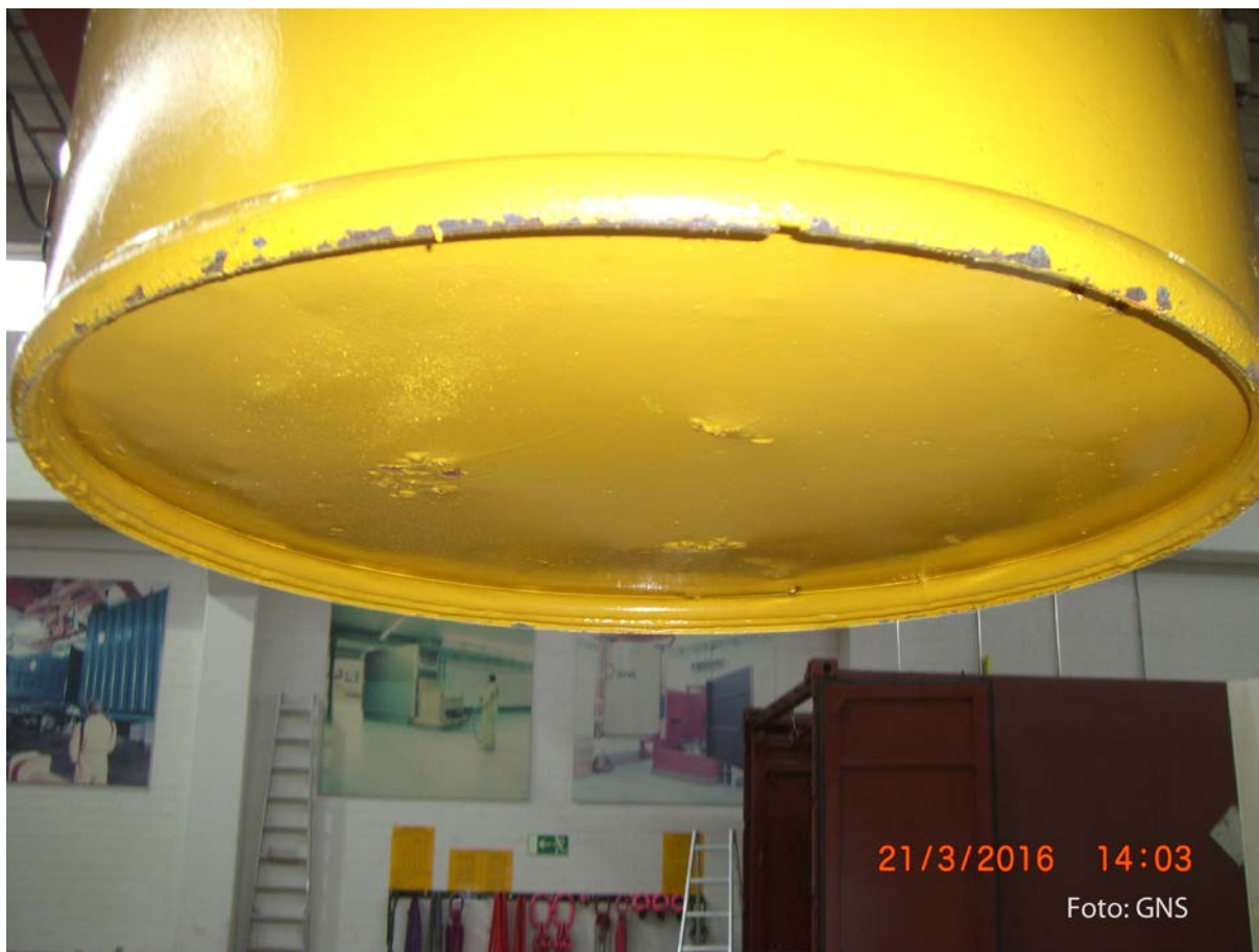
Fig.1: Examples of corrosion at Gorleben, Lower Saxony, (Photo: GNS)
